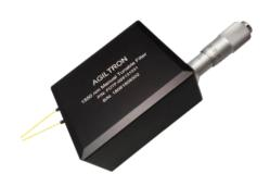
Agiltron's Manual Grating-Based Fiber Optic Tunable Filter provides a simple way to adjust the center wavelength of narrow band over wide band. Wavelength tuning is achieved by rotating a grating using a micrometer.
